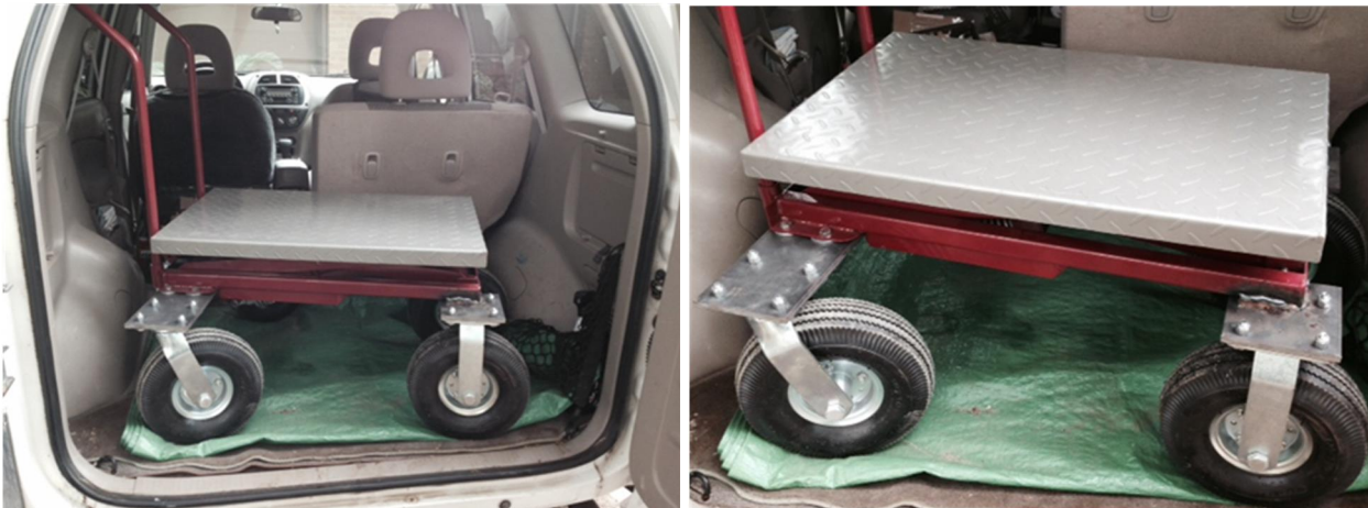
The After - New wheels, wider improved balanced footprint, Iteration 3
